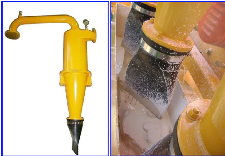
Illus.: Hydro vacuum cyclones
