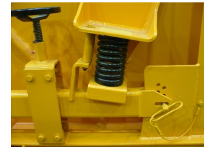
III. 2: Screen Angle adjustment
