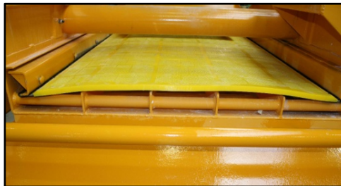
III.: Hook-strip screen (Upper deck)
