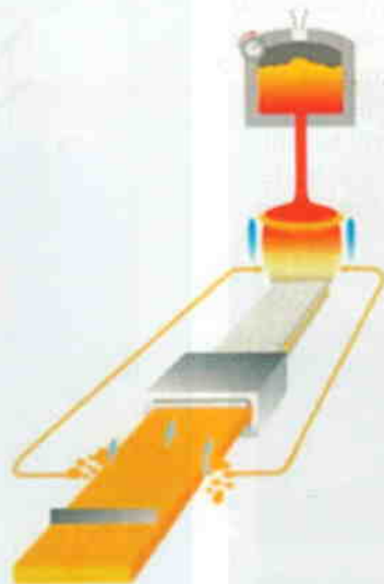
Production of glass wool from the melting chamber up to cutting out
