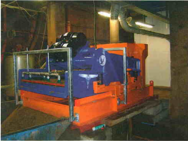
2 ITE Siebmaschine 3PSM • Screening machine 3PSM from ITE
